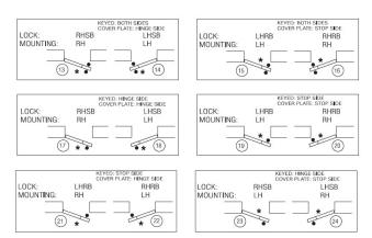
\* Indicates lock mounting/access plate side.
